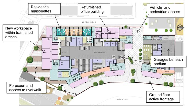
Figure 22: Annotated ground floor layout plan
