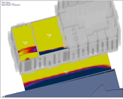
Figure 28: Model showing shadows cast over Islay Wharf
